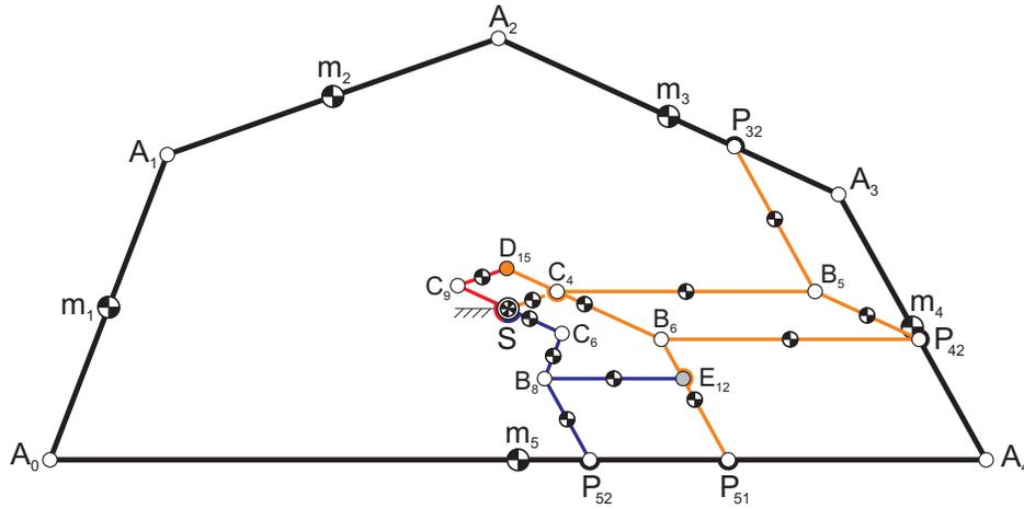
**Figure 7.** Normally constrained inherently balanced linkage solution where  $S$  is the common CoM of all 17 links for any of its 3-DoF motions.
