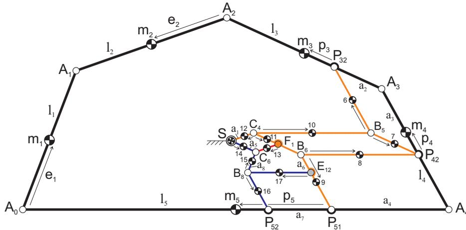
**Figure 8.** Inherently balanced linkage solution of Fig. 7 with modification for compactness, obtaining a similar five-bar linkage  $B_8C_6F_1B_6E_{12}$ , with the link mass parameters included.
