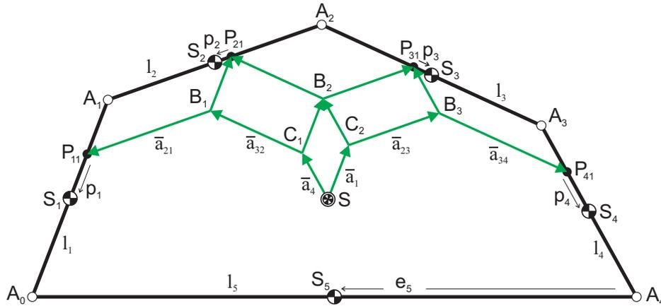
Figure 1. 5R Five-bar linkage  $A_0A_1A_2A_3A_4$  with system of principal vectors defining the common CoM in  $S$ .
