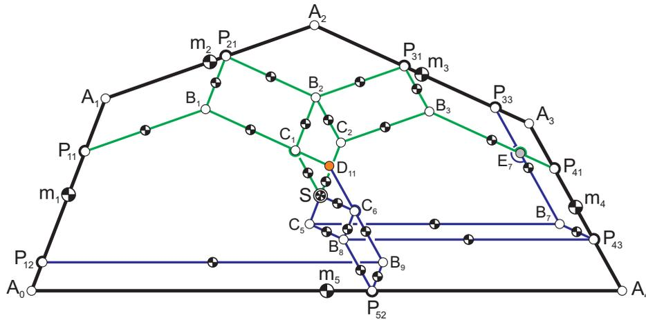
**Figure 4.** Five-bar linkage with two sets of principal vector links based on two not neighboring systems of principal vectors together with their interconnections.
