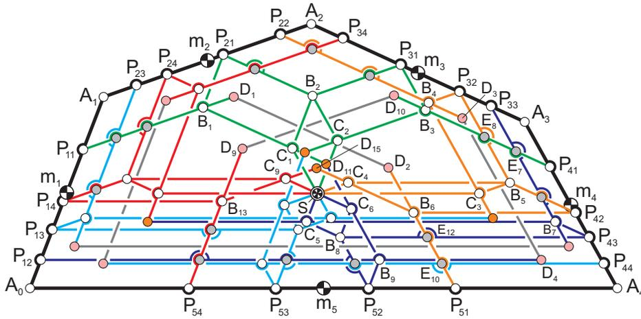
**Figure 5.** Grand 5R Five-bar-based Inherently Balanced Linkage Architecture with 65 links, 58 overconstraints, and 3-DoF motion with joint  $S$  as the common CoM of all links.
