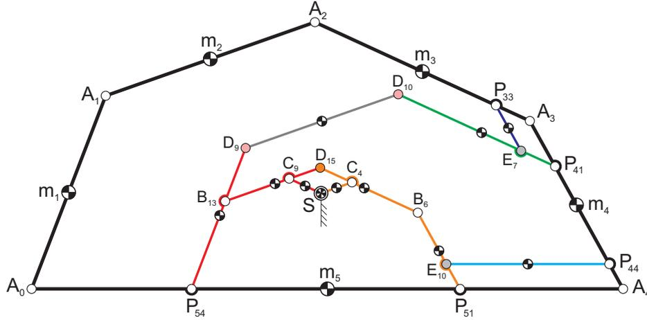
**Figure 6.** Normally constrained inherently balanced linkage solution where  $S$  is the common CoM of all 15 links for any of its 3-DoF motions.
