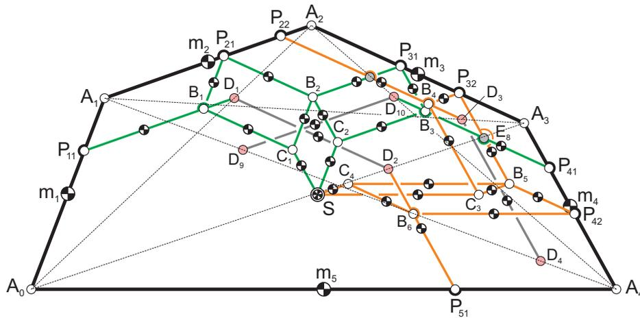
**Figure 3.** Five-bar linkage with two sets of principal vector links based on two neighboring systems of principal vectors together with their interconnections.
