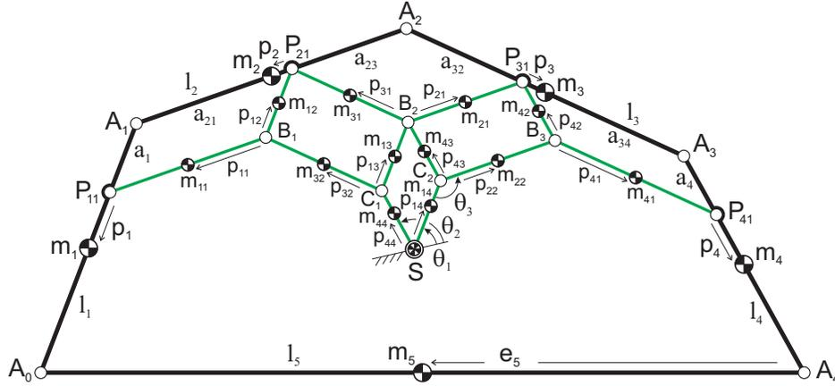
**Figure 2.** 3-DoF closed-chain principal vector linkage with the common CoM of the 17 links in  $S$  for any of its motions. With  $S$  as fixed base joint the linkage is force balanced with respect to the base.
