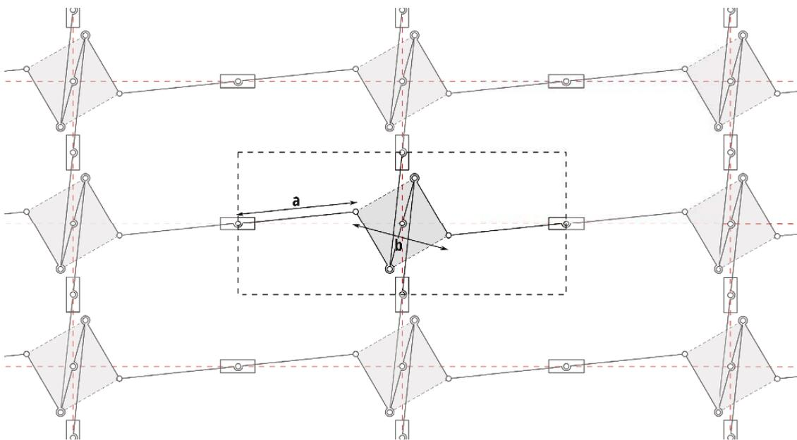
**Fig. 4.** Proposed design of a periodic linkage with a Poisson's ratio of 1 based on inversor linkages. Red dashed lines indicate the slider paths. The central unit cell of the linkage is indicated with a dashed black line. The gray squares indicate rigid bodies which have a pivot at the intersection of the horizontal and vertical slider paths. The diagonals of the grey squares have length  $b$  and the four bars have length  $a$ .
