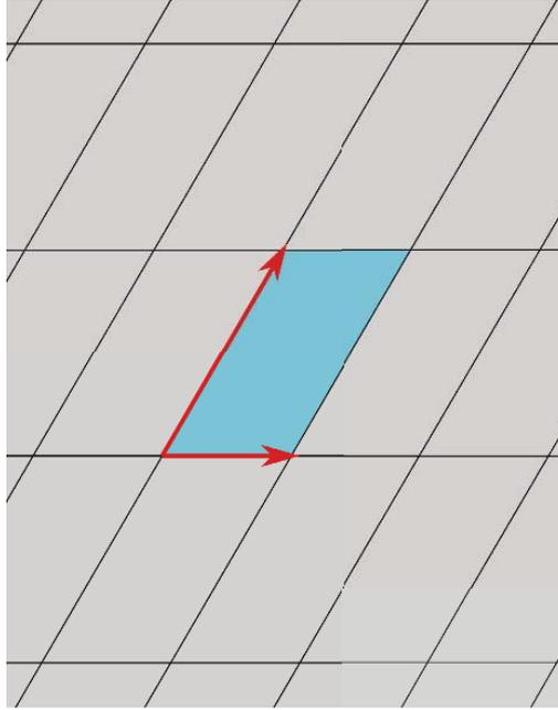
**Fig. 1.** A periodic linkage consists of a unit cell (highlighted in cyan) which is copied along two non-parallel vectors (red arrows) to fill the plane. Within this unit cell, a linkage is constructed with periodic boundary conditions, maintaining connectivity between neighboring unit cells.
