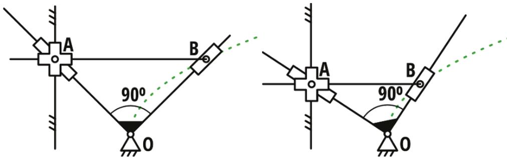
**Fig. 6.** Antonov's Parabolograph in two different configurations. Point  $O$  is fixed to the ground, point  $A$  is fixed to a vertical line. When actuated, Point  $B$  moves along a parabolic path, indicated by the green dotted line. Figure adapted from Fig. 215 in Artobolevskii's book [18]
