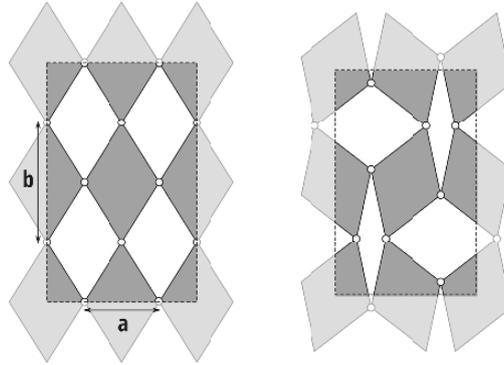
**Fig. 2.** Four pantographs can be combined to form a unit cell with  $\nu = -1$ . The grey plates are rigid and allowed to hinge at their corners. The unit cell is indicated by a dashed line. This structure is adapted from [11].
