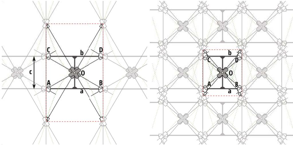
**Fig. 7.** Proposed design of a periodic linkage based on Antonov's Parabolograph with a constant Poisson's ratio of  $-\frac{1}{2}$ . Two different configurations are shown. The unit cell is indicated by a dashed red line, the corners of this unit cell follow the green dashed parabolic paths. The points  $A, B, C$  and  $D$  slide over lines  $a$  and  $b$ . Point  $O$  is situated at the center of the unit cell. The two crossed bars pivot around this point.
