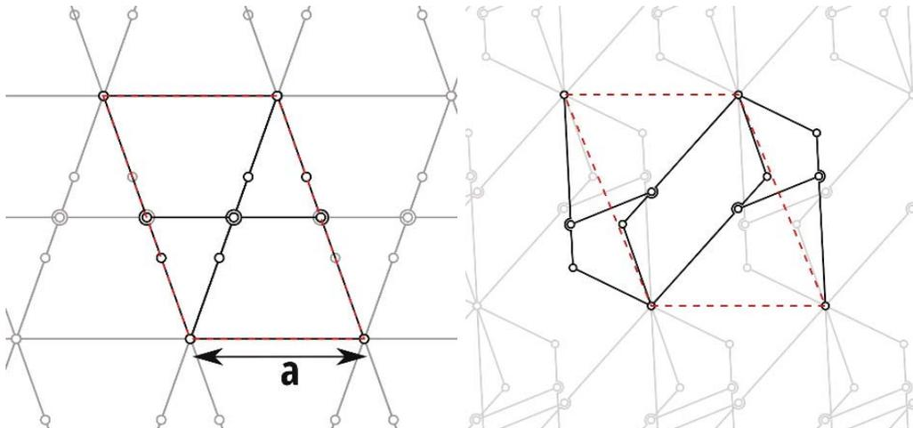
**Fig. 5.** Proposed design of a periodic linkage with  $\nu = 0$ , based on Hart's A-frame. Shown are two configurations within its range of motion. The unit cell is indicated by the red dotted line and drawn with black lines, The rest of the lattice is drawn in gray. When this linkage moves, the height of the unit cell decreases, but its width remains the constant distance  $a$ .
