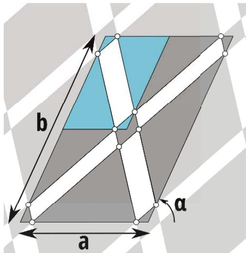
**Fig. 3.** Proposed design of a planar parallelogram-shaped unit cell, we can construct a set of four pantograph linkages, merged together such that there is one degree of freedom for the mechanism which corresponds to  $\nu = -1$ . The gray faces in this drawing are rigid elements and connected by revolute joints at their corners. The pantograph in the upper left corner is highlighted.
